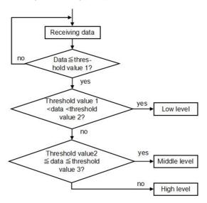
Fig. 4. Process of force data acquisition
