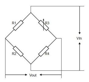
Fig. 3. Working principle of TH4805 sensor
